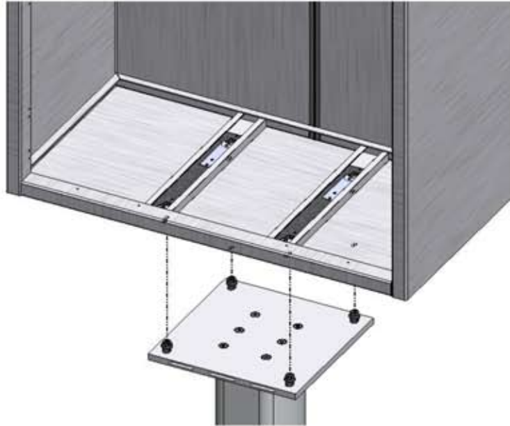
Figure 16 – Removing Cabinet from Pedestal
