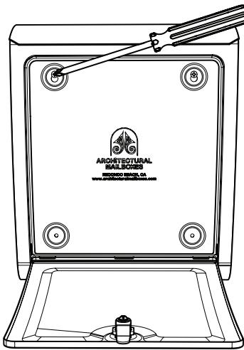
**5** While the mailbox is hanging on the top screws, insert the remaining two screws into the bottom holes and secure with a screwdriver.
